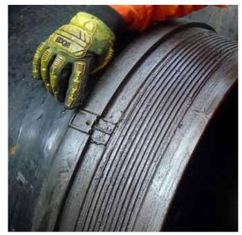
ARKs: Pre-installed at the mill, housed and bolted with no loose parts and no need for special equipment make activation really quick and simple, taking just a few seconds.
