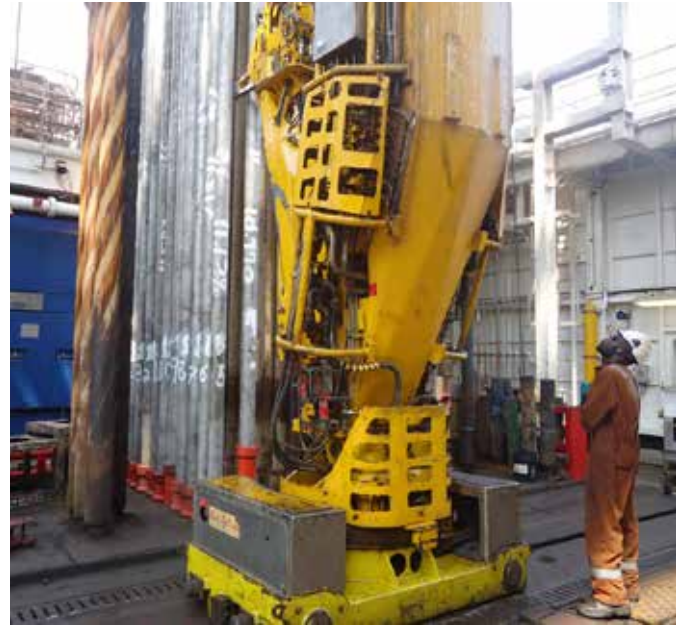
▲ Running CRAs with Dopeless® connections in triples made the operation 62.5% faster and efficient.
